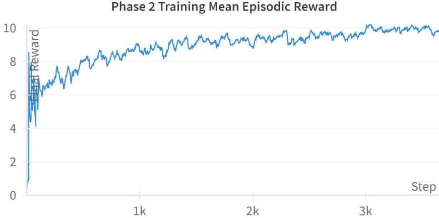
Figure 4.11: Average episodic total reward curve for Phase 2. Note that direct comparison with Phase 1 is not feasible due to the episode length being halved from 20 secs to 10 secs.
